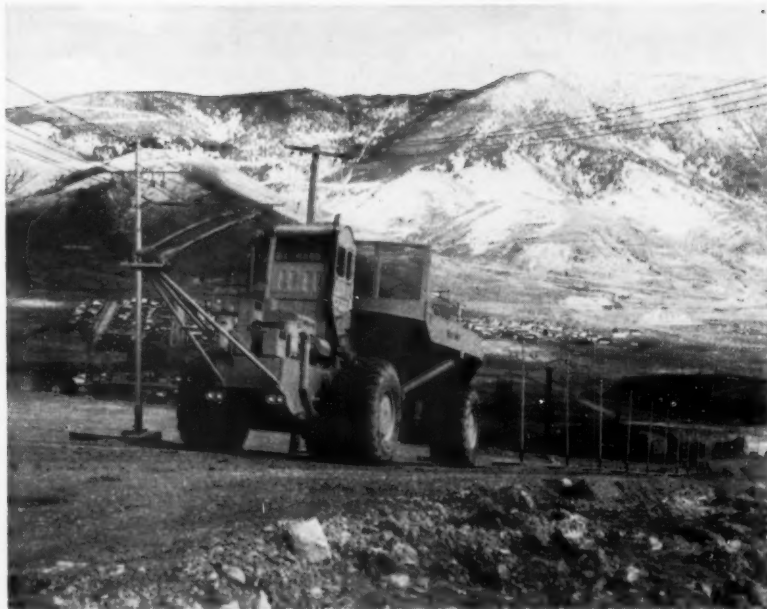
TRUCK hauls up to 75 tons of Berkeley pit waste up a 15 percent adverse grade at a speed of 12 miles per hour—about double the speed of Diesel haulage.
